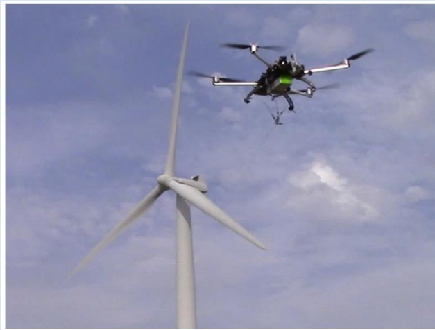
A remotely controlled quadcopter carries a temperature-sensing fiber-optic cable to investigate atmospheric mixing in an active wind farm. Credit: Robert Predosa
