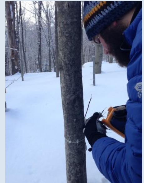
Hand-logged and data-logged snowpack temperature profiles ground to 1 m at 10 cm intervals; 1 min resolution
